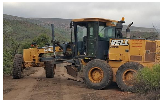
Figure 17: Example where grader drives off the road to make a u-turn or get out of the way of oncoming traffic.
