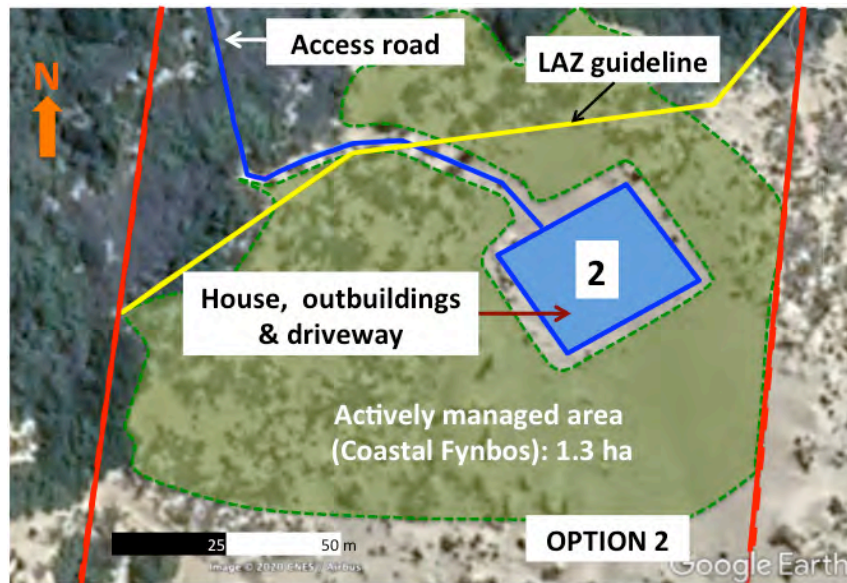
Figure 16b: For Option 2 an area of 1.3 ha surrounding the dwelling is actively gardened to form a coastal fynbos interface to prevent wind-blown sand inundation off the blow-out on the dune top.
