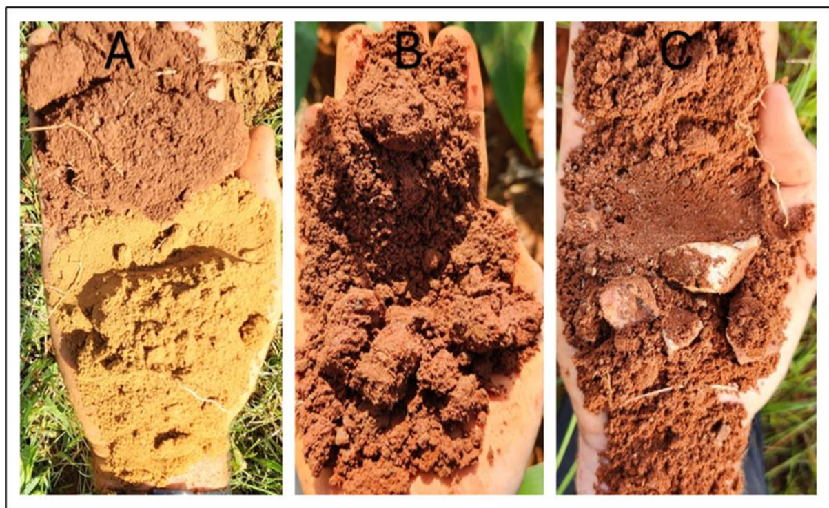
Figure 3-3 Soil forms and diagnostic horizons identified on-site: A) Ermelo soil form (Orthic/ Yellow-brown horizon); B) Red apedal subsurface horizon from Hutton soil forms; C) Glenrosa soil form.
