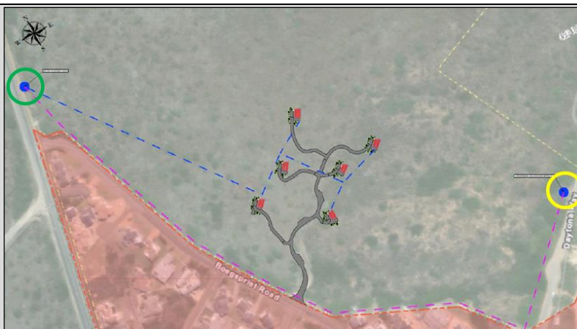
Figure 16: Rising water line (purple line) from the borehole (yellow circle) to a 10kl water reservoir (green circle) from where water will be gravity fed to the six pods (blue line) (Source: Element Engineers).
