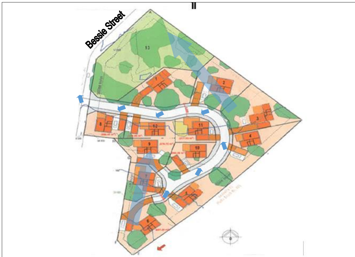
Figure 7: Stormwater drainage on the internal street will be designed to drain into Bessie Street. The site generally drains overland towards a northern and north-western direction.
