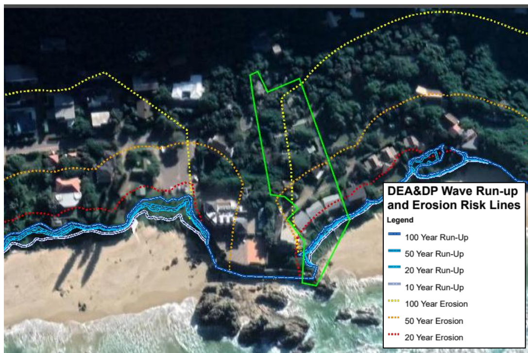
Figure 10: DEA&DP Eden District wave run-up and erosion risk lines at Keurboomstrand
