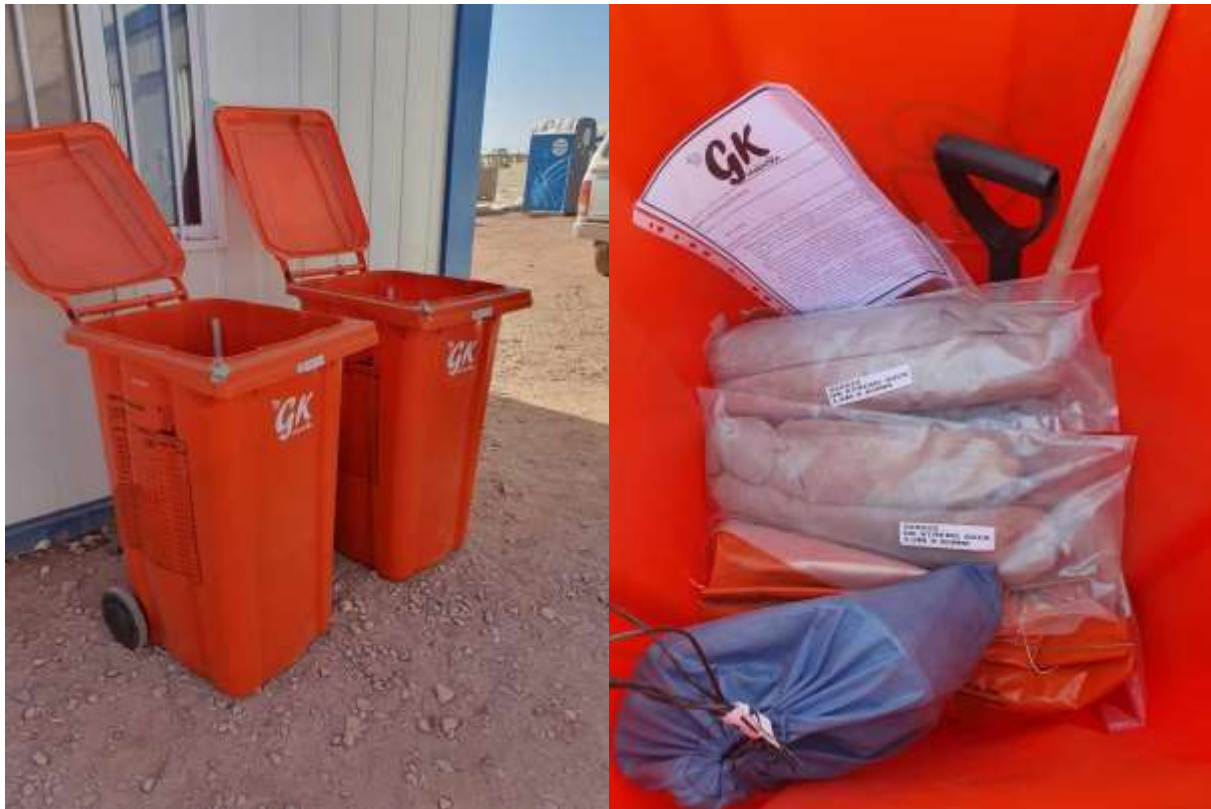
Figure 6: Hydrocarbon Spill Kits must be in place within the site camp and in the field within 500m of any excavation activity.
