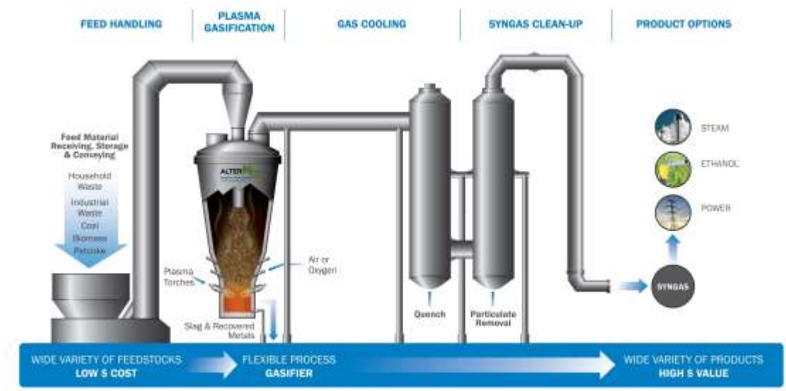
Figure 32: Biomass gasification (WPP Energy Corp, 2010)
