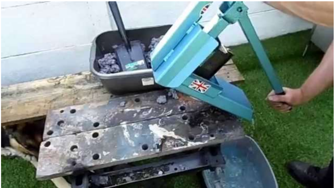
Figure 9: Manual briquette maker (Source: Multimate Designs)
