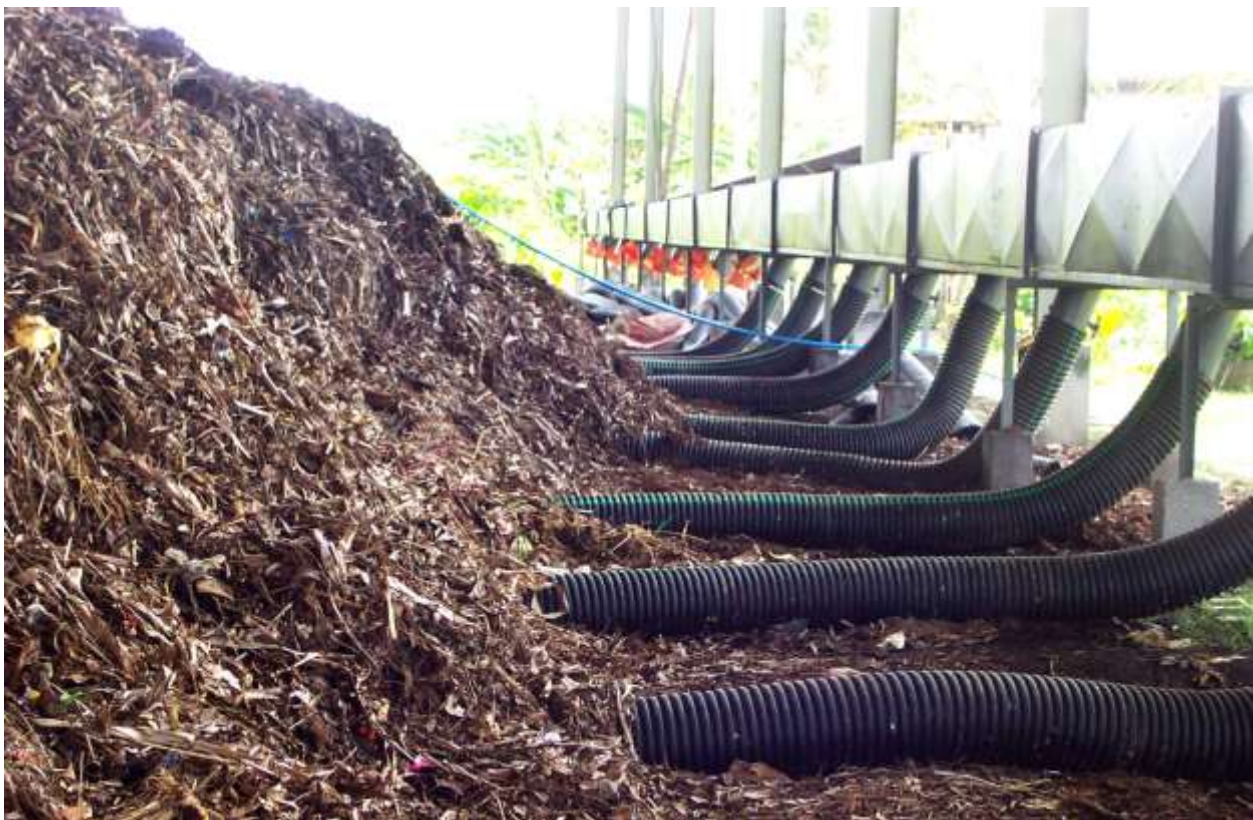
Figure 24: The biomass is aerated to ensure aerobic composting, resulting in the production of carbon dioxide and heat rather than methane (myclimate, 2017)
