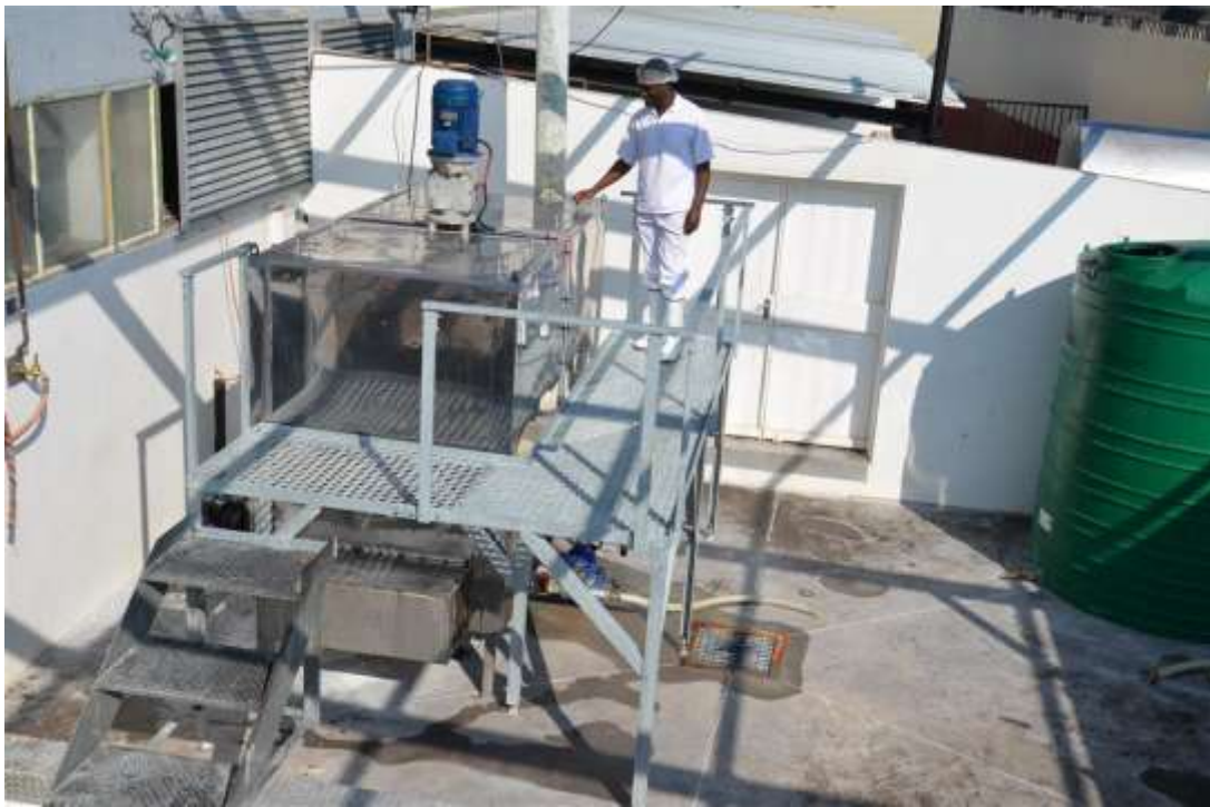
Figure 38: Micro rendering plant outside of an abattoir (WRT, 2017)
