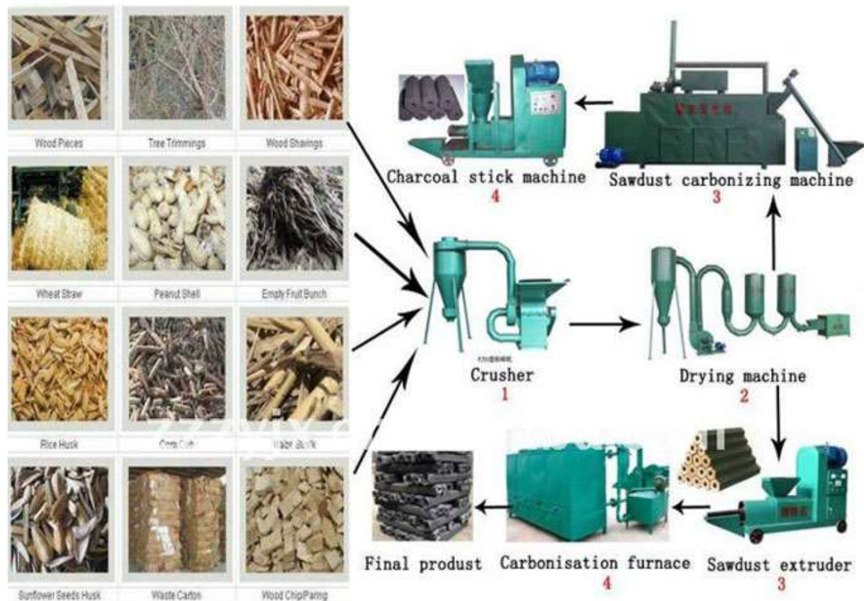
Figure 8: Mechanised briquette maker (Source: Kefan Machinery)
