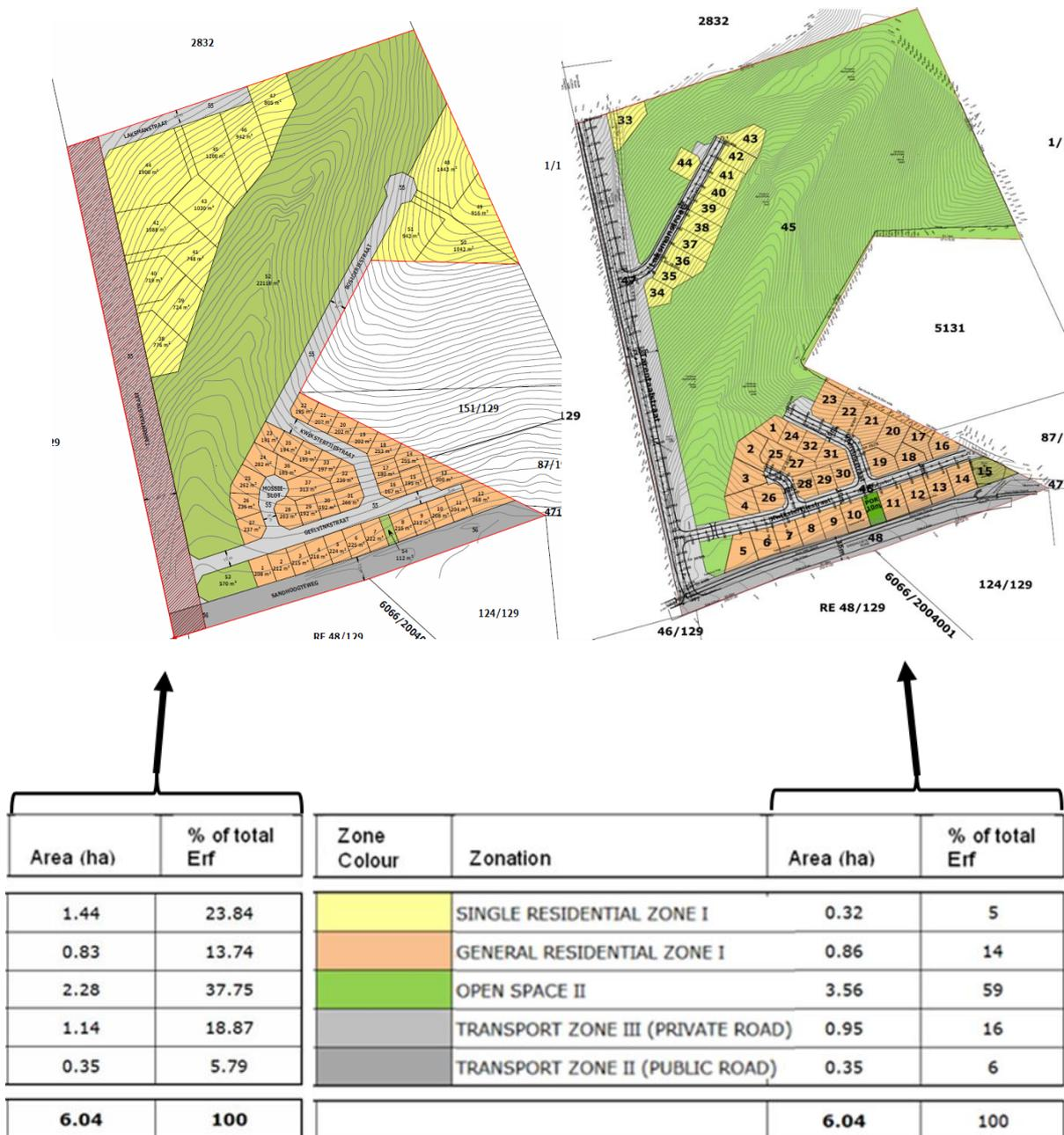
Figure 2: The two proposed site development plans (SDPs) for Erf 2833. On the top left is the non-mitigated alternative plan, and the top right is the preferred alternative SDP. The zonation categories are given below the SDP maps.
