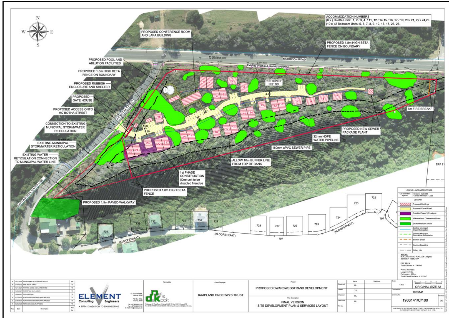
Figure 13. The proposed development layout for the northern development area of Erf 610, Dwarswegstrand. The green shading shows the locations of sensitive trees that would be retained.
