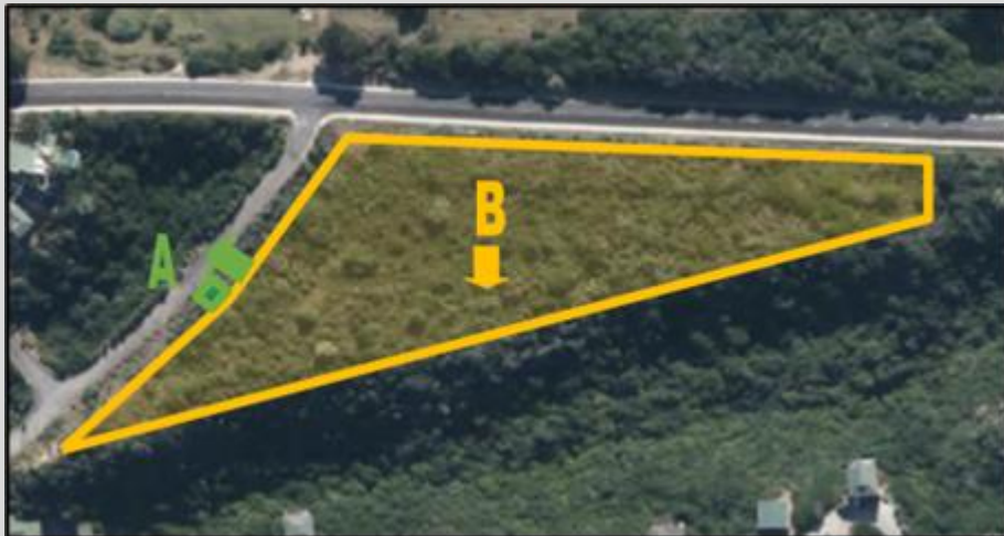
Figure 8: Direction of stormwater drainage with a minor percentage (~5%) towards H.C. Botha (Position A) and the rest (~95%) will infiltrate and be handled on-site (Position B).
