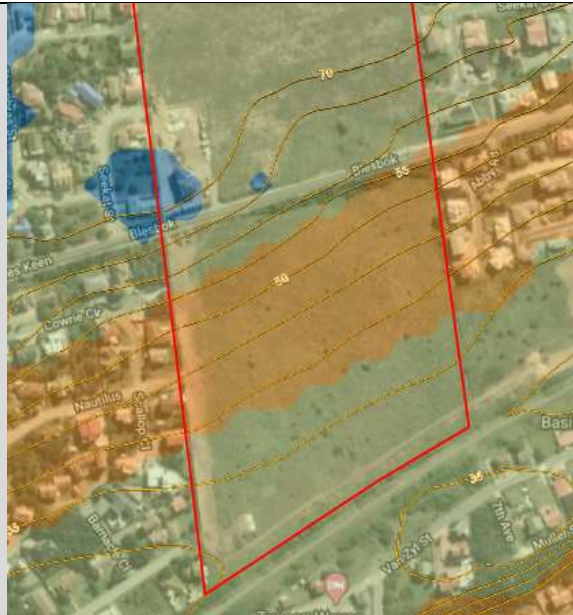
Figure 13: Slope analysis for the study site indicating the steepest part of the site (orange).
