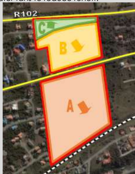
Figure 9: Stormwater drainage catchments for the study site (Source: Element Engineers 2019).
