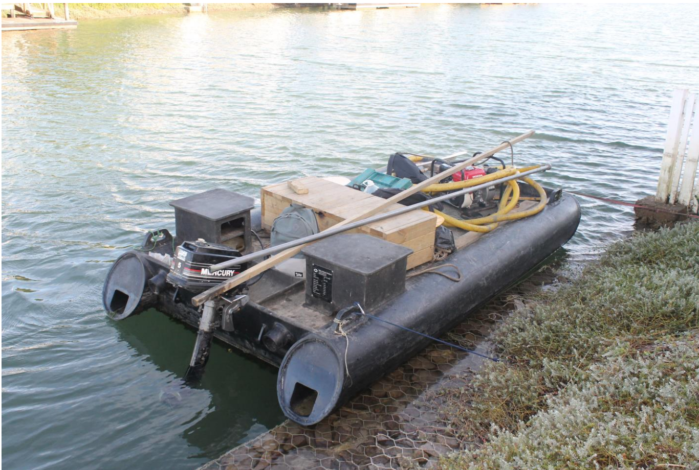
Figure 17: Example of the barge used to conduct visual inspections and remove/replace jetty structures (high water jet visible on barge).
