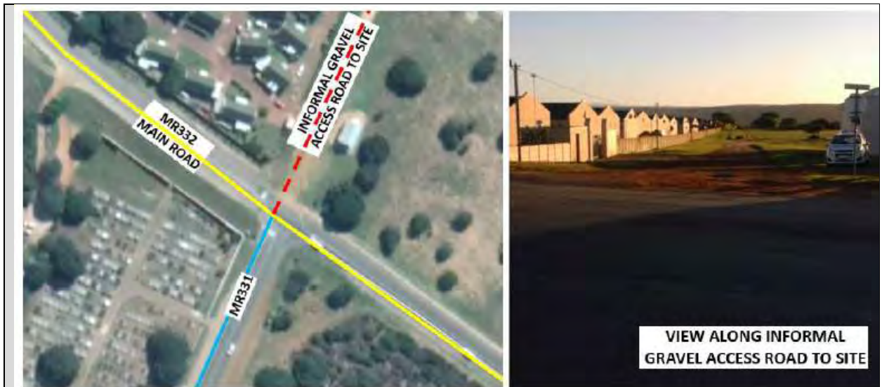
Figure 7: Left aerial image indicates the MR331/MR332 intersection, as well as the informal access to the site. Right side photo is a picture of the existing informal access off Main Road that will be upgraded as access road and feed into the 4-way stop at MR331/MR332.
