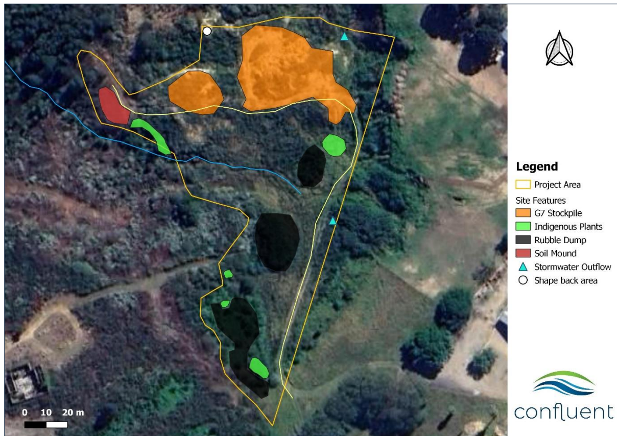
Figure 2. Relevant features present at the site which form part of the MMP.
