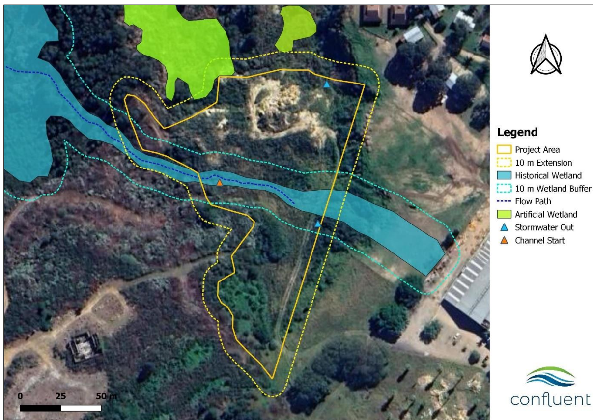
Figure 10. Historical wetland area indicating 10 m buffer either side, and 10 m extension area (if necessary) around the Project Area.
