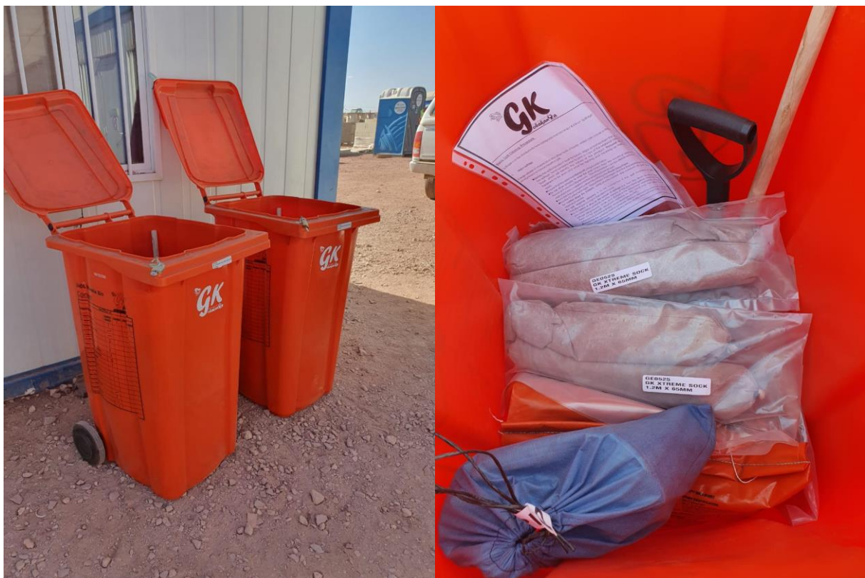
Figure 4: Hydrocarbon Spill Kits must be in place within the site camp and in the field within 500m of any excavation activity.
