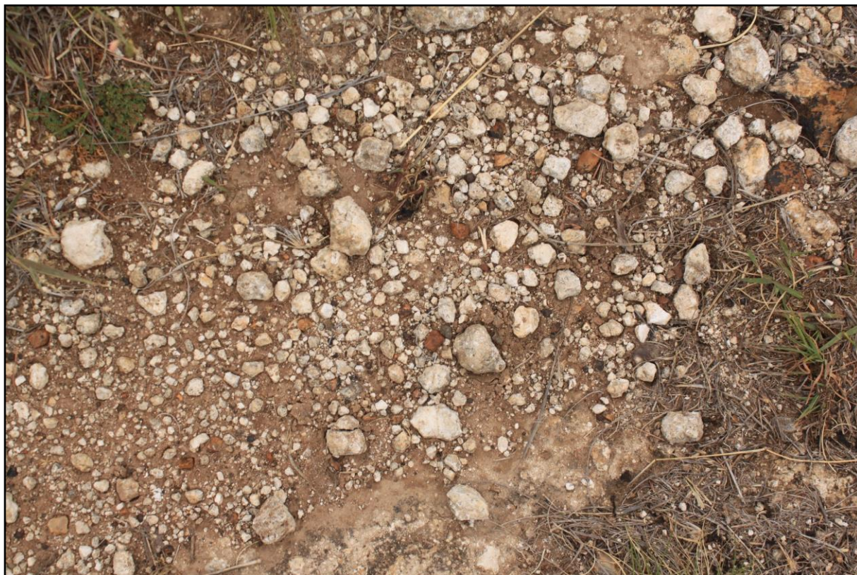
Figure 7: Coega soils within the grid assessment corridor with nodules of hard carbonate visible on the surface
