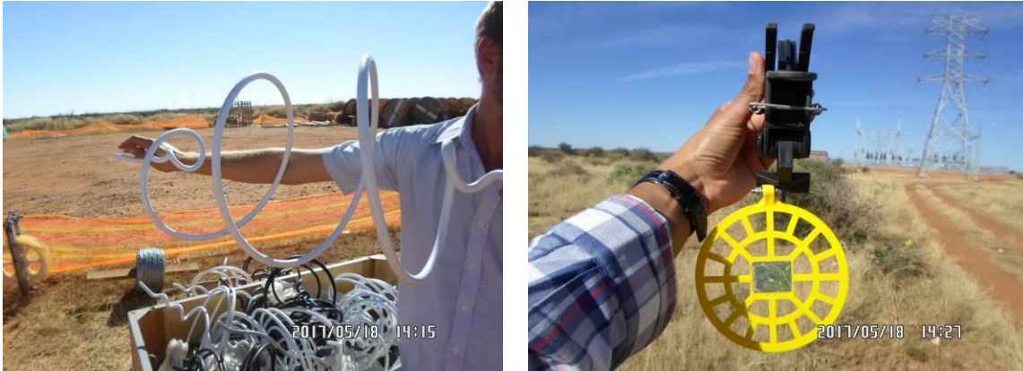
Figure 20: Examples of bird flight diverters to be used on the power lines: Double loop bird flight diverter (left) and Viper live bird flapper (right).
