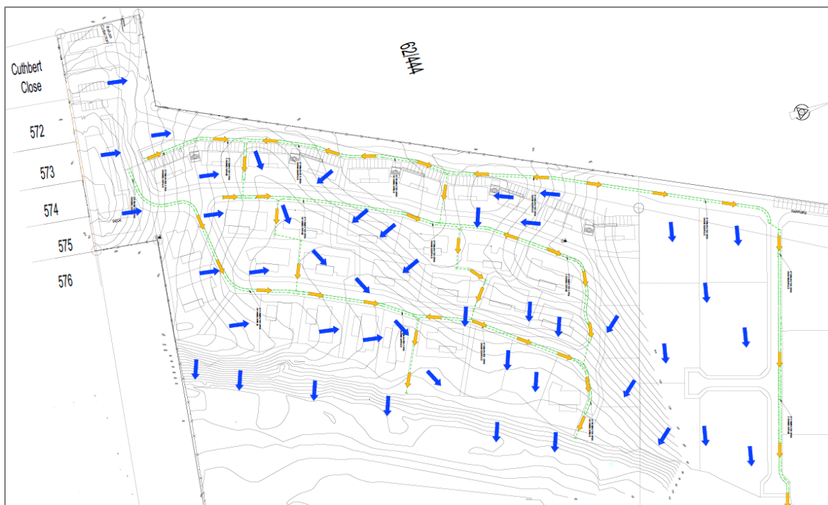
Figure 7-1: Overland drainage patterns
