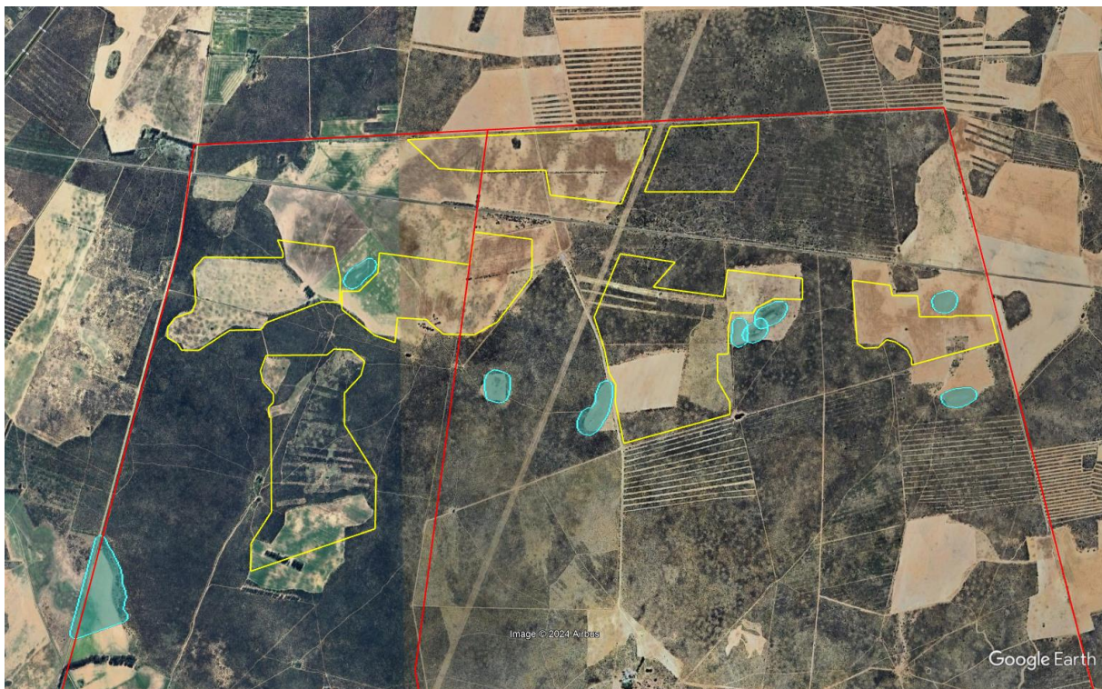
Figure 45: Showing how the aquatic features and their associated buffers have been avoided by the mitigated preferred alternative (Layout Alternative 5).
